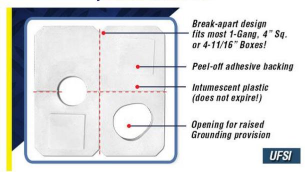
Peel-off adhesive backing -- Openings for ground emboss / pigtail -- Fits 4" Sq., 4-11/16" Sq. and 1G switch boxes -- Intumescent plastic - does not expire! -- Never use putty to fire-rate a box again! -- Convenient to Prefab -- STC rating of 52 -- Rated for 2hr wall assemblies
